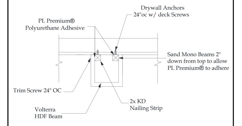
HDF Beams which weigh more than 3.25 lbs per L/F - cleating, blocking or nailing strip shall be glued, screwed and mechanically fastened to structural members—check local codes before installing beams. Distance between blocking not to exceed Volterra's written recommended span for HDF Beams - typical is 2" x 6" @ 24" on center. Nailing strip to be continuous.
