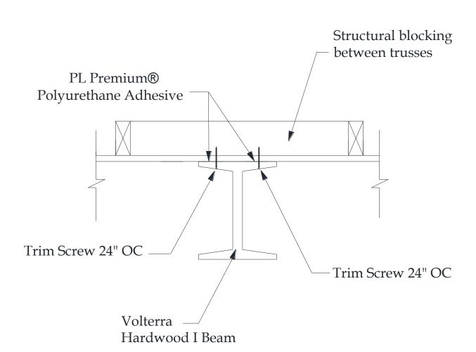
Volterra I Beams must be glued to drywall with PL Premium urethane construction adhesive. Apply 2 continuous 1/4" beads on top of beam. Mechanically fasten beams 24" OC with Trim Screws (predrill holes for screws) to structural blocking above drywall. Patch screw holes if necessary with wood putty and touch up paint. Check local codes before installing beams.
