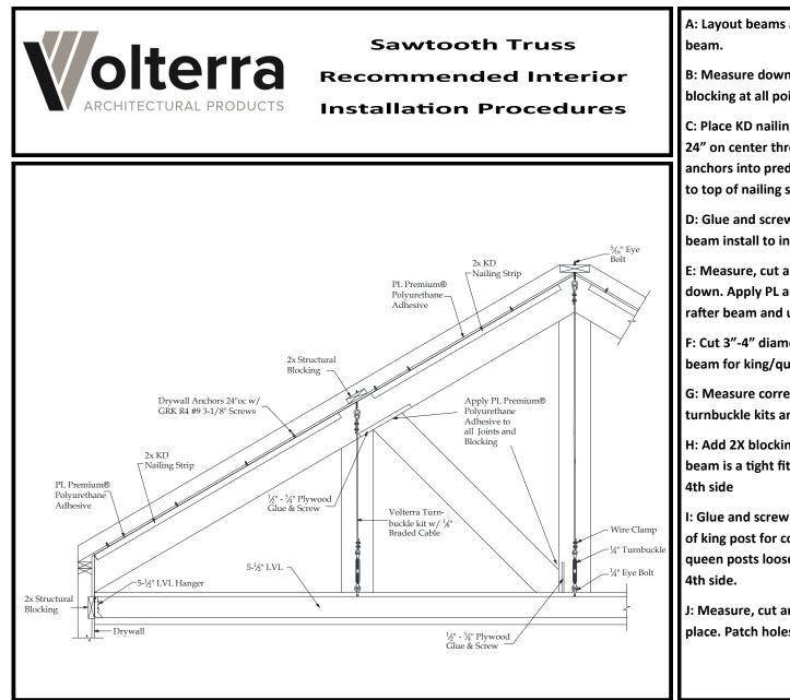
A: Layout beams and chalk lines to the inside of rafter beam.
