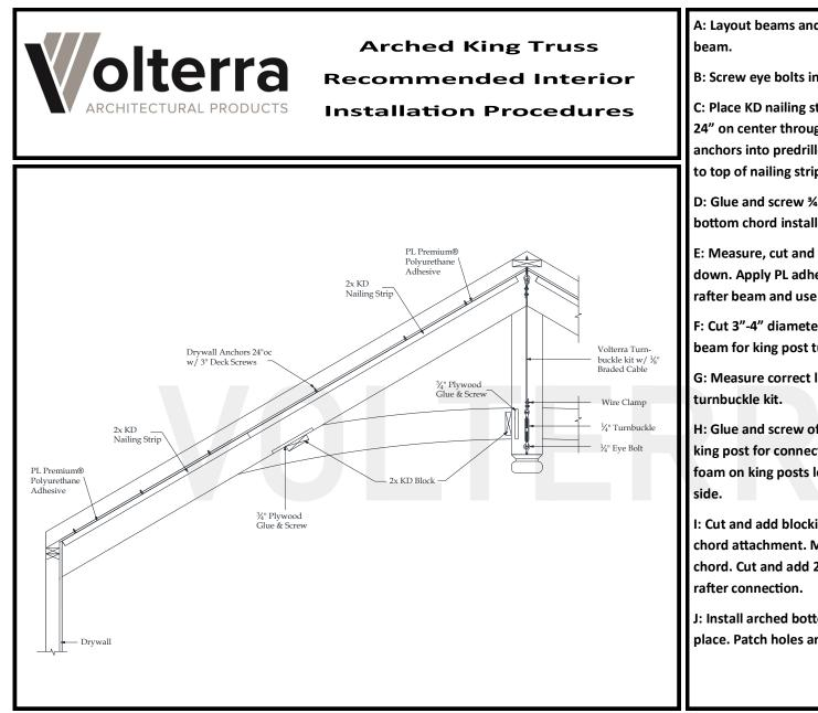
A: Layout beams and chalk lines to the inside of rafter beam.
