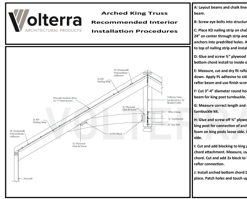
A: Layout beams and chalk lines to the inside of rafter
