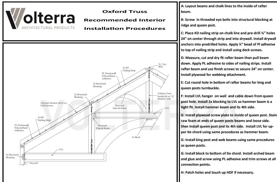
D: Measure, cut and dry fit rafter beam then pull beam down. Apply PL adhesive to sides of nailing strips. Install rafter beam and use finish screws to secure 24" on center.
