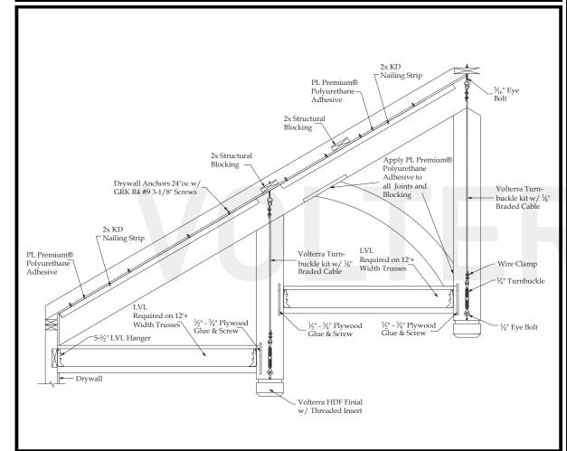
A: Layout beams and chalk lines to the inside of rafter beam.
