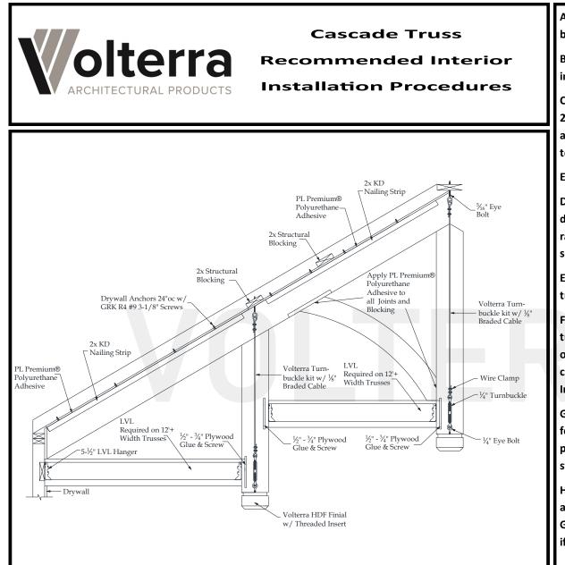
A: Layout beams and chalk lines to the inside of rafter beam.
