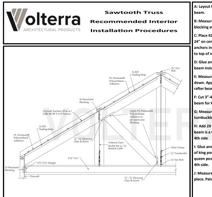
A: Layout beams and chalk lines to the inside of rafter beam.
