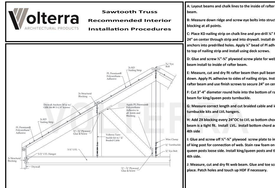
B: Measure down ridge and screw eye bolts into structural
